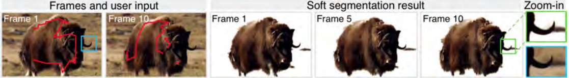
Figure 5.16: Failure case of proposed video object segmentation algorithm. Left: Two frames with red foreground scribbles. Right: Soft segmentation result. Zoom-ins: Result ( top ), input ( bottom ). Copyright of original video: Discovery Communications.
