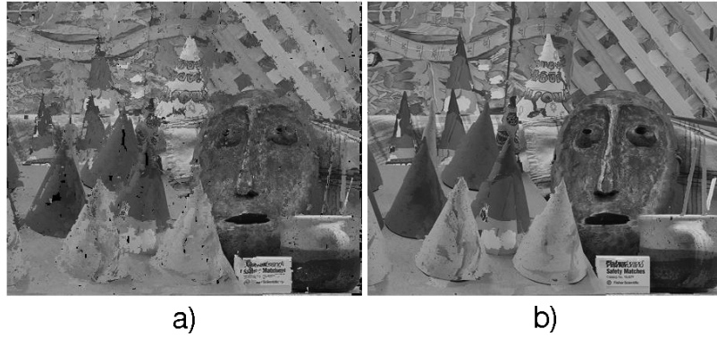
Figure 6: Interpolation results to generate novel views. a) Shows the novel view after the initial search for corresponding blocks. It contains holes (black). The final results after the refinement steps are shown in b).
